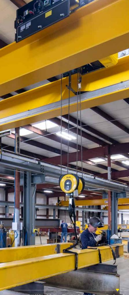
Engineered Systems chose R&M's NRGmaster energy chain which enhances the cranes' headroom by removing the traditional festoon and placing the track inside the web of the bridge beam, giving the cranes an overall cleaner appearance, and protecting the wires from accidental contact with equipment or objects in the area.
