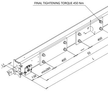
The wheel loads listed are only a guideline. The max. wheel load listed is based on the structural integrity of the frame and load placement, and it does not take into account permissible wheel loading or bearing life. SG load placement is at the center, and DG load placement is for a trolley gage of 1200 mm [47 1/4\*].
