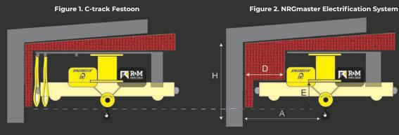
Potential space savings when using R&M's QX cranes (Figure 1) and the added space savings versus standard C-track festoon system cranes
