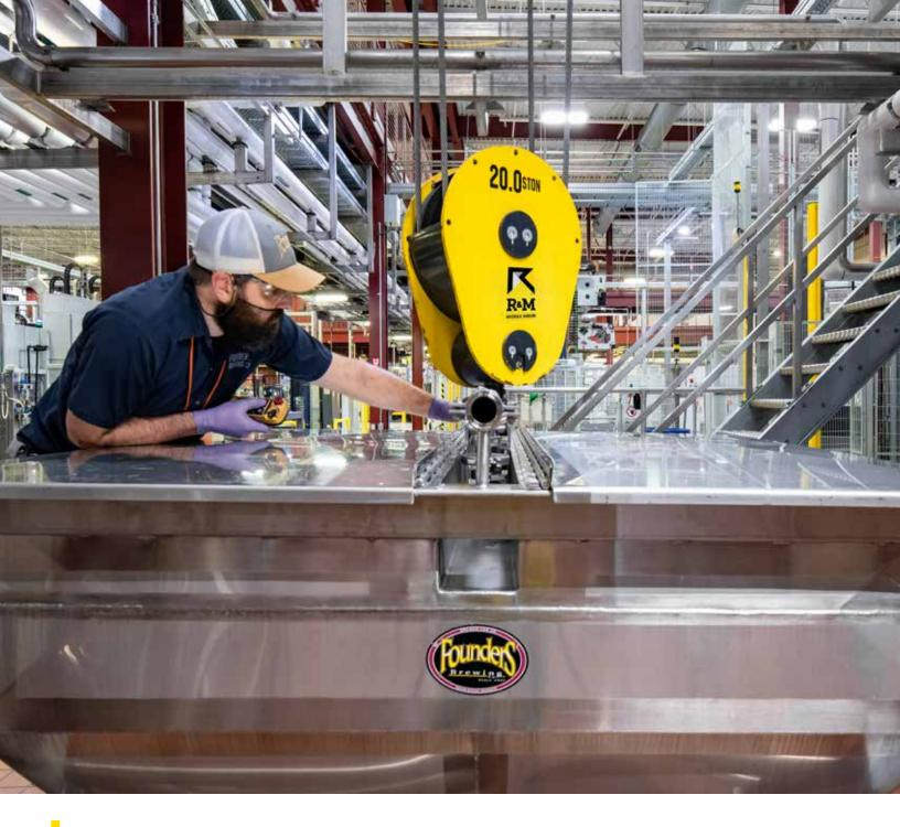
"We chose this route specifically to perform the task of dry hopping profusely that we are known for. We didn't want to choose the common solution of pumping the hops in the tank, nor a 'hop cannon'. We wanted to drop the hops in the top of the tank and designed the crane specifically to do this."
