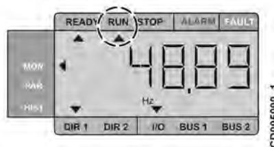
The drive status is located above the LCD display. The status of the drive is indicated with different states:
