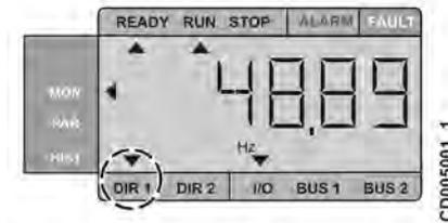
The control selections are located below the LCD display. The control selections:
