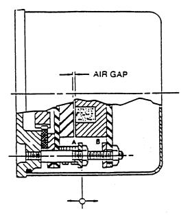
MOVE THIS DIRECTION TO INCREASE TORQUE AND PROVIDE QUICKER STOP. MOVE THIS DIRECTION TO REDUCE TORQUE AND PROVIDE SMOOTHER STOP.
