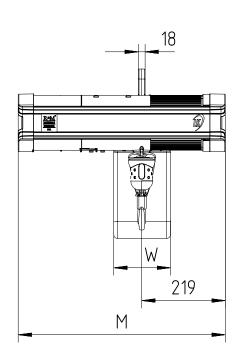
Note: In case of 2-fall hoist, hook suspension is rotated by 180°.
