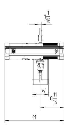
Note: In case of 2-fall hoist, hook suspension is rotated by 180°.
