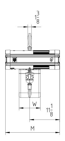
Note: In case of 2-fall hoist, hook suspension is rotated by 180°.
