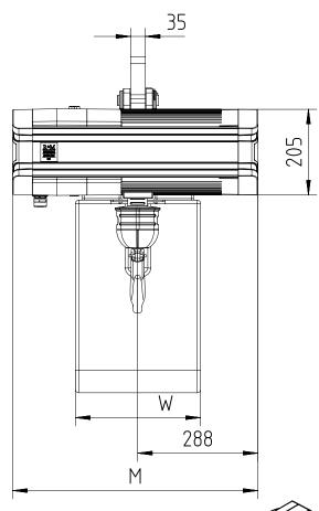
Note: In case of 2-fall hoist, suspension eye is rotated by 180°. Note: Add 60mm to C & L dimension for hoisting speeds greater than 8 m/min.
