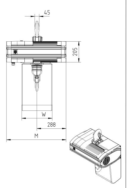
Note: In case of 2-fall hoist, suspension hook is rotated by 180°. Note: Add 60mm to C & L dimension for hoisting speeds greater than 8 m/min.
