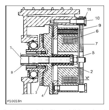
If maximum air gap of brake has been reached or will be exceeded before next inspection, readjust air gap.
