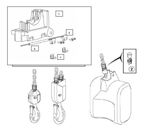
Table 13. Chain Guide Assembly with Limit Switches Parts List
