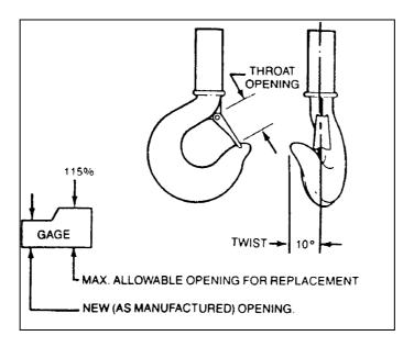
Due to many types and sizes of hooks that can be furnished and/or specified by the user / owner, it is recommended that user / owner measure the actual throat opening of hook as originally furnished. See *Figure 20*. Record the throat dimension on above sketch. Retain as a permanent record. This record can then be used for determining when hook must be replaced due to deformation or excessive throat opening.
