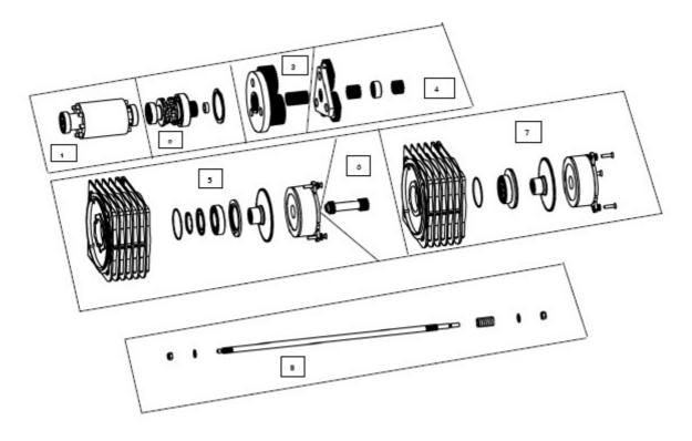
Table 14. Double Brake Mechanism Parts List
