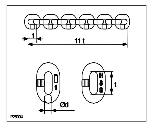
Measure the following chain dimensions at several points on chain: (Figure 13)
