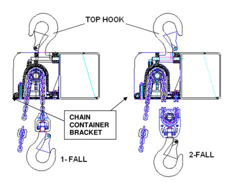
CAUTION: Before removing Top Hook, de-energize the power to the hoist per ANSI Z244.1 and make certain that any load is removed from the load hook. Also support the total weight of the hoist, including chain, prior to removing the Top Hook.
