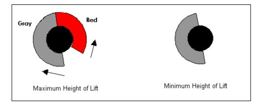
To reset the rotary limit once it has tripped, the load block assembly must travel approximately 11" [27cm] in opposite direction.
