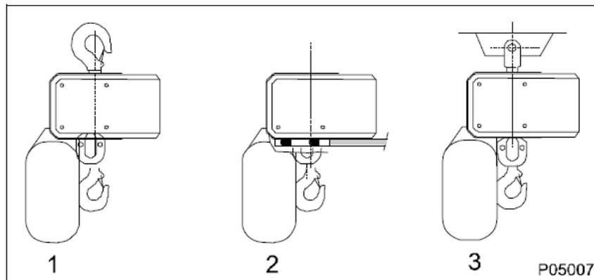
For all trolley-mounted hoists, refer to appropriate trolley manual for trolley installation instructions.
