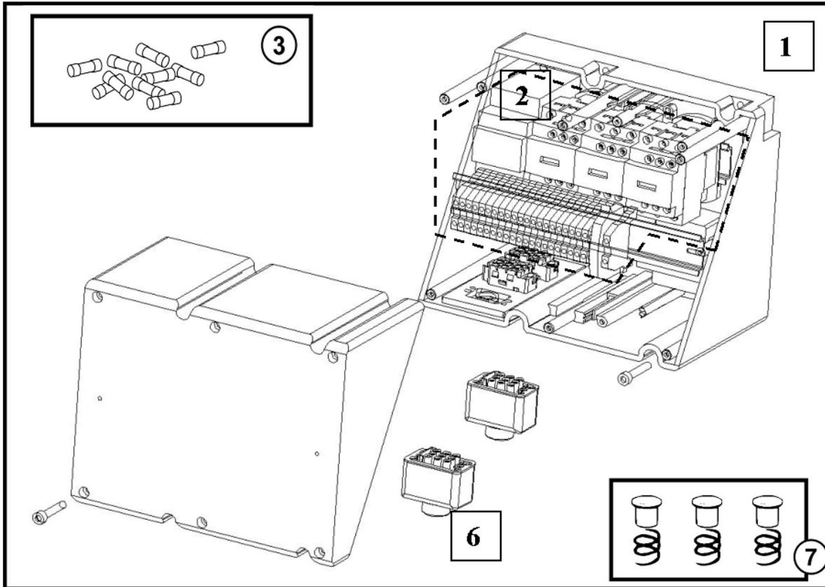
Table 16. C16/C20/C25 Electrical Control Assembly Parts List
