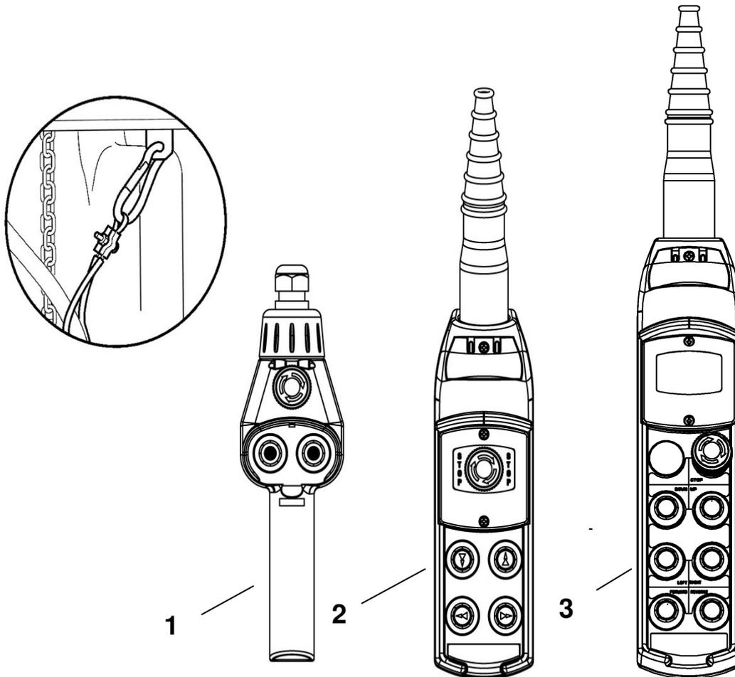
Table 20. Push Button Assembly – Horizontal Pairs of Buttons Parts List
