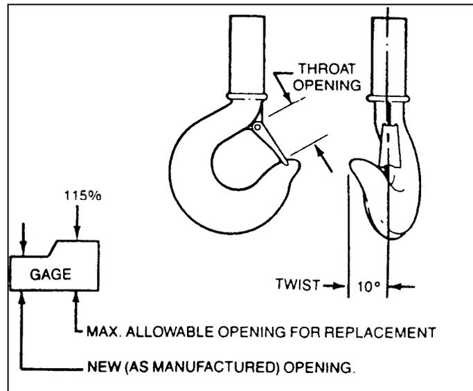
Due to many types and sizes of hooks that can be furnished and/or specified by the user / owner, it is recommended that user / owner measure the actual throat opening of hook as originally furnished. See *Figure 16*. Record the throat dimension on above sketch. Retain as a permanent record. This record can then be used for determining when hook must be replaced due to deformation or excessive throat opening.
