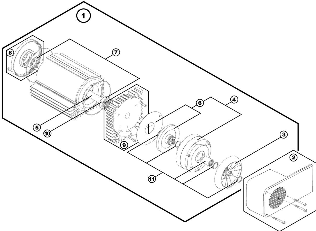
Table 13. C16/C20/C25 Hoist Motor and Brake Assembly Parts List
