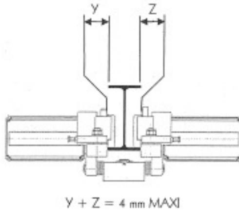
Adjust drive wheel and idler wheel/side plates as shown above.
