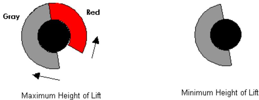
**To reset the rotary limit once it has tripped, the load block assembly must travel approximately 11” [27cm] in opposite direction.**
