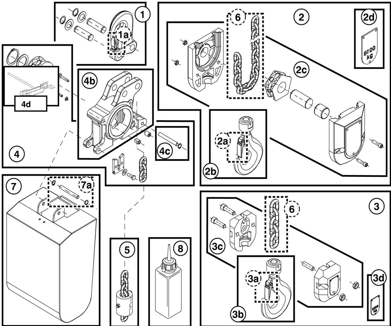
Table 15. C20 / C25 Lifting Assembly Parts List - (C20 / C25 ONLY)
