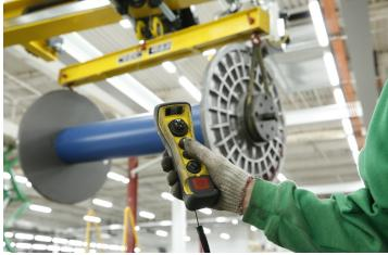
While HSI installed an NRGmaster at Everest Textile with 2-ton capacity, Mike said he's used the crane in heavier industry applications because it can be ordered with a capacity up to 80 tons. The NRGmaster can also accommodate two hoists per bridge beam and, Mike said, it's quiet.
