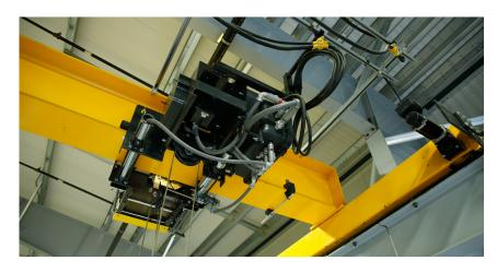
Like the Spacemaster SX, the EX features an innovative design that includes a large drum diameter, which enables both the lowest headrooms and best wheel loads in the industry, while providing near-true vertical lift with single reeving. Employing a large diameter drum also makes it possible for exceptional hook approaches and lift heights.
