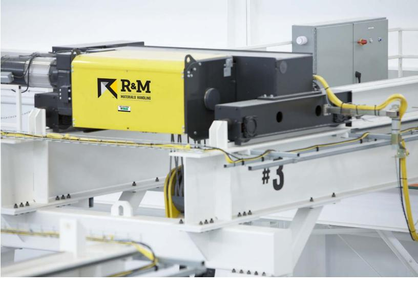
Wolverine constructed the cranes with pre-engineered components from R&M Materials Handling, Inc., and from controls supplier Drivecon, Inc. The integrated package plays an important role in the assembly process of the wind turbine nacelles, adds Kelps. The hoists, one per work-cell, lift the nacelle structure and/or its component parts to assist in that stage of assembly.
