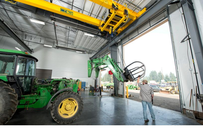
The crane, which has been operational since January 2018, incorporates custom lasered girder connection side plates and an enclosed track conductor bar, which permitted only 9 in. of horizontal cope in the beam. It is the only crane in the building and it serves the three northern bays (four, five, and six) of the workshop. This floor coverage increased the value of the crane and lowered the initial cost owing to a shorter length runway system.
