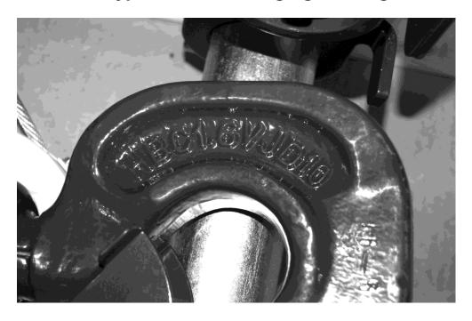
An example of markings on an HBC1.6V size load hook.
