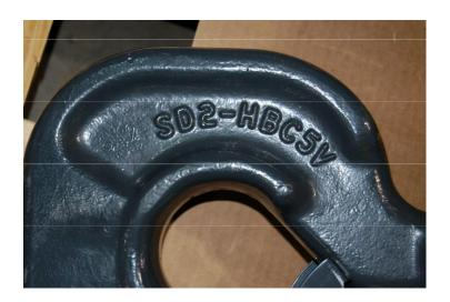
An example of markings on an SD2-HBC5V size load hook.
