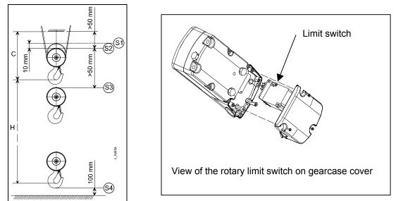
Headroom is dimension C and lift is dimension H. Total reach is headroom + lift (C+H).
