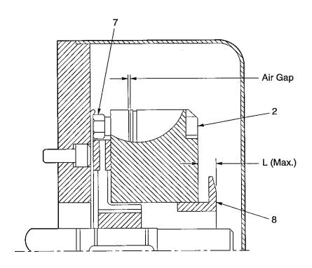
The brake is adjusted for proper torque when shipped from the factory and should not require adjustment in the field. If necessary, torque rating can be reduced by unscrewing torque adjustment ring (8) with a spanner tool. The torque adjustment ring has detent action with a torque reduction per step as indicated in chart below.
