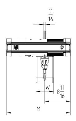
Note: In case of 2-fall hoist, hook suspension is rotated by 180°.
